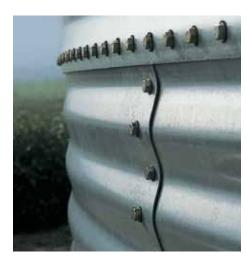
**Strong sidewall sheets** feature 4-inch (102-mm) corrugations. In addition, each BROCK® Sidewall Sheet is 44 inches (1118-mm) wide which reduces erection costs because the bin goes up faster.
