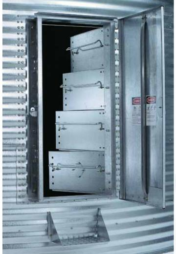
Industry-leading bin accessories like Brock's LATCH-LOCK® Walk-Through Bin Door make grain storage manageable with the least amount of hassle. The one-piece outer door opens wide to fasten securely against the side of the bin. The four interlocking inner panels open in sequence from top to bottom with a simple lift of the patented latches. No tools required.
