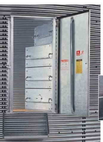
Industry-leading bin accessories like Brock's LATCH-LOCK® Walk-Through Bin Door make grain storage manageable with the least amount of hassle. The one-piece outer door opens wide to latch securely against the side of the bin. The four interlocking inner panels open in sequence from top to bottom with a simple lift of the patented latches. No tools required.
