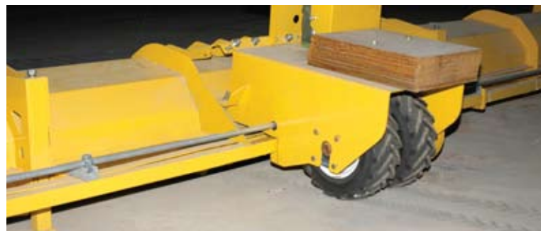
Sweep Drive with Foam-Filled Dual Wheels
